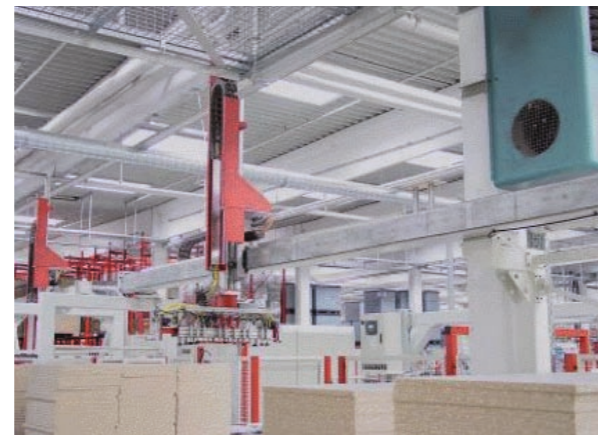
2-axis gantry with universal tooling
