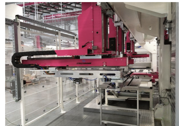
Feeder for blank handling
