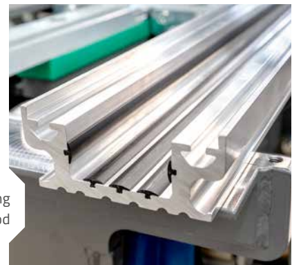
Floor cut-out for the holding profile
